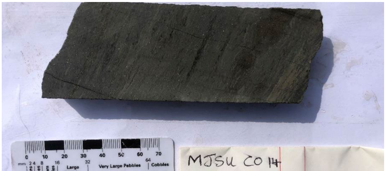
MJSU 14 (MJSU Co 14), MMAJ "Black Mud" - finely banded tuff with abundant laminated pyrite and other very fine-grained sulphide minerals. MMAJ interval 220.20 - 220.90m, 0.24 g/t Au, 34.0 g/t Ag, 1.13% Cu, 35% Zn, and 1.2% S.
